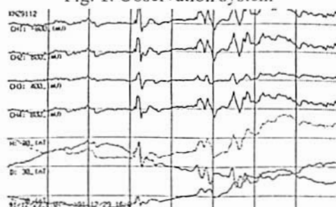
Fig.3. Example of obtained data. Upper four channels are geoelectric records. The numbers of the channels correspond to the numbers shown in Fig. 2. Lower three channels are geomagnetic records obtained at Kakioka.
